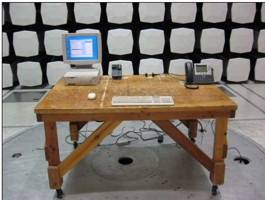
Photograph 2. Conducted Emissions Test Setup, Mode 2
