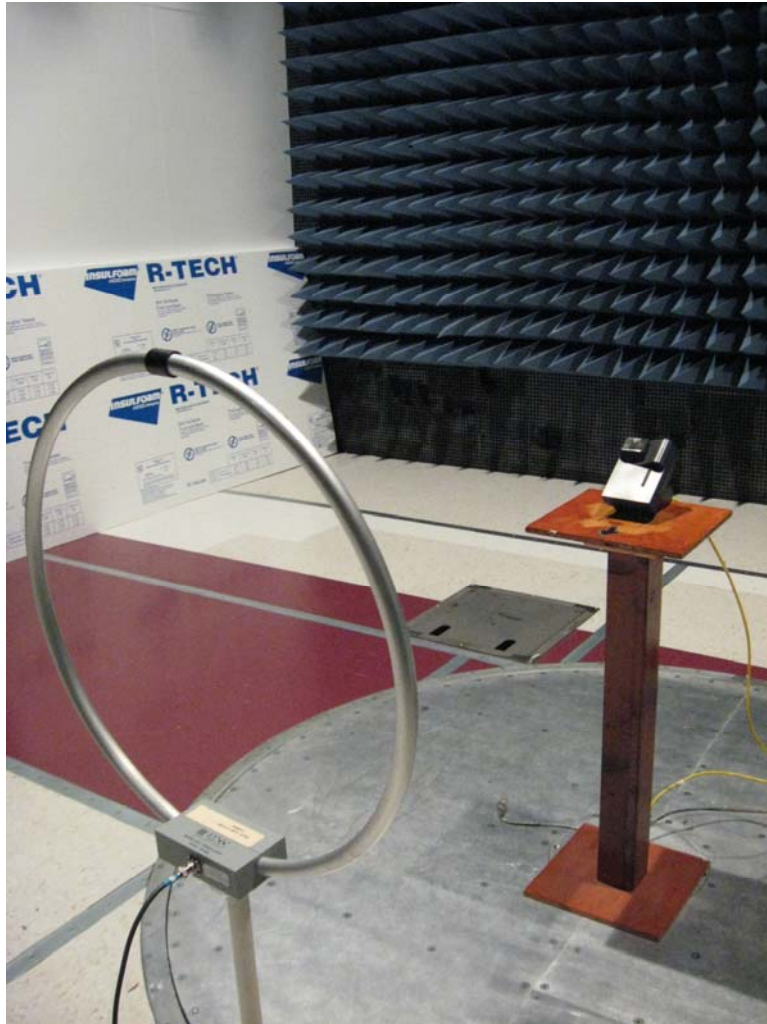
Photograph 5. Measurements below 30 MHz
