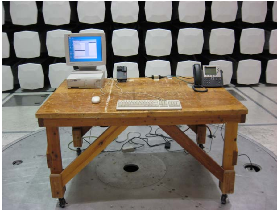
Photograph 1. Conducted Emissions Test Setup (AC Power Brick)
