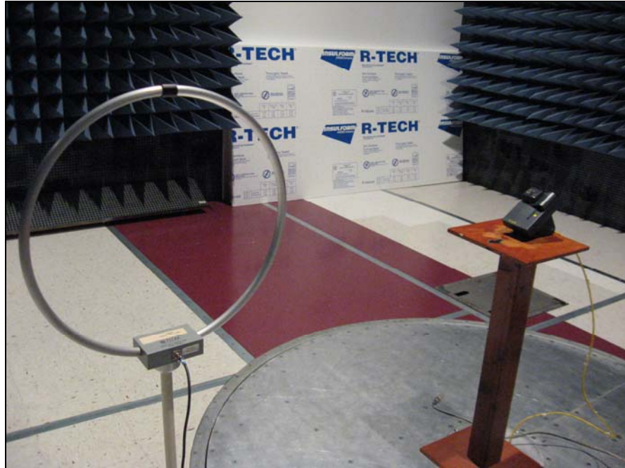
Photograph 4. Measurements below 30 MHz
