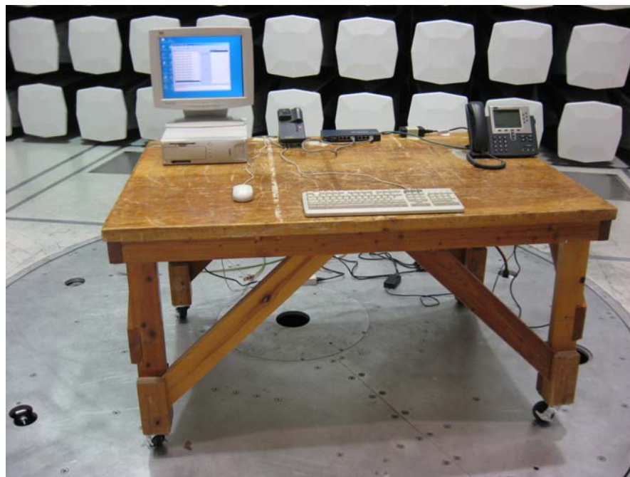
Photograph 2. Conducted Emissions Test Setup (POE)
