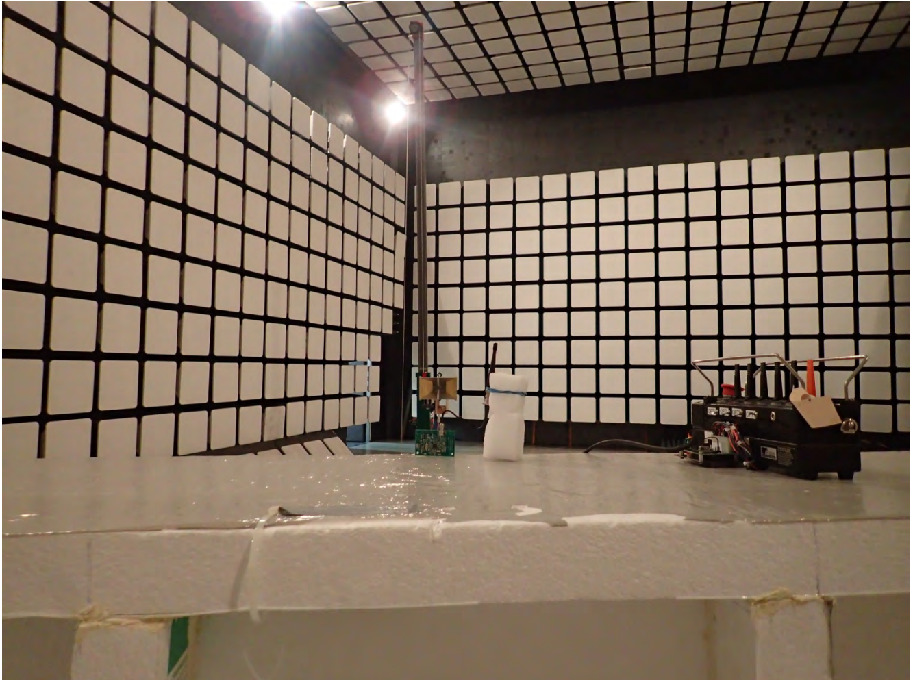
Radiated Emissions @ 3 m EUT with Laird EXC902BNX Antenna, Orthogonal Position 2
