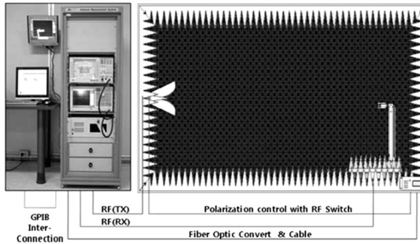
Chamber - MTG 6x3x3(m), 300MHz~6GHz
