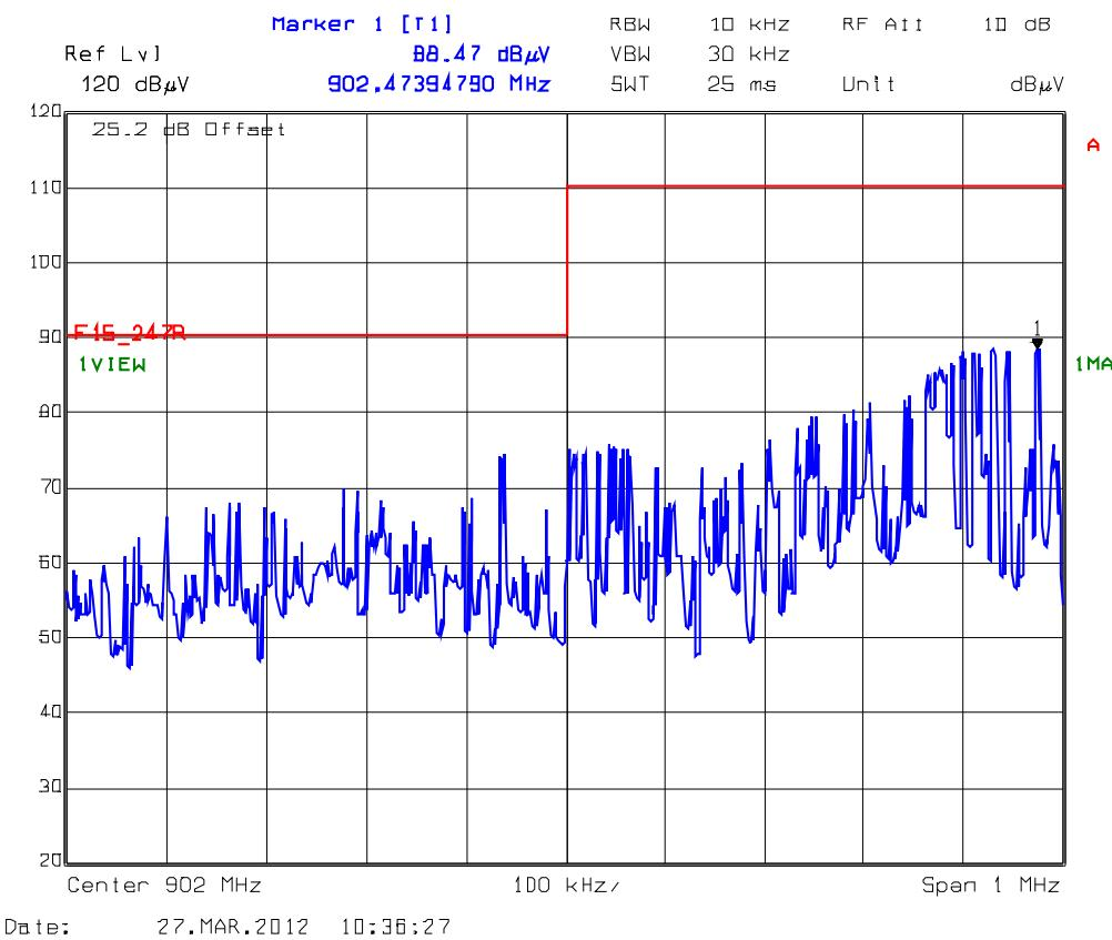
Lower Band Edge with Hopping Function ON
