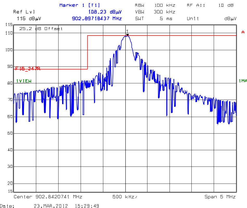
Lower Band Edge with Hopping Function ON
