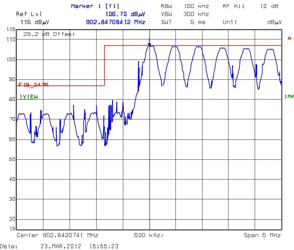
**Plot 5.10.4.1.2 Lower Band-Edge RF Radiated Emissions @ 3 meter
