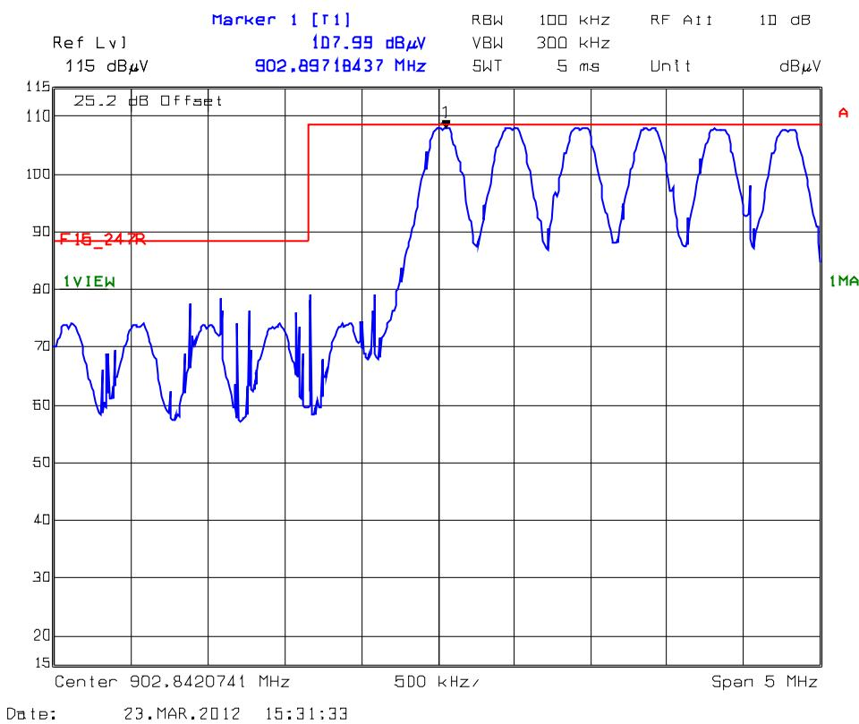
**Plot 5.10.4.1.3** Upper Band-Edge RF Radiated Emissions @ 3 meter
