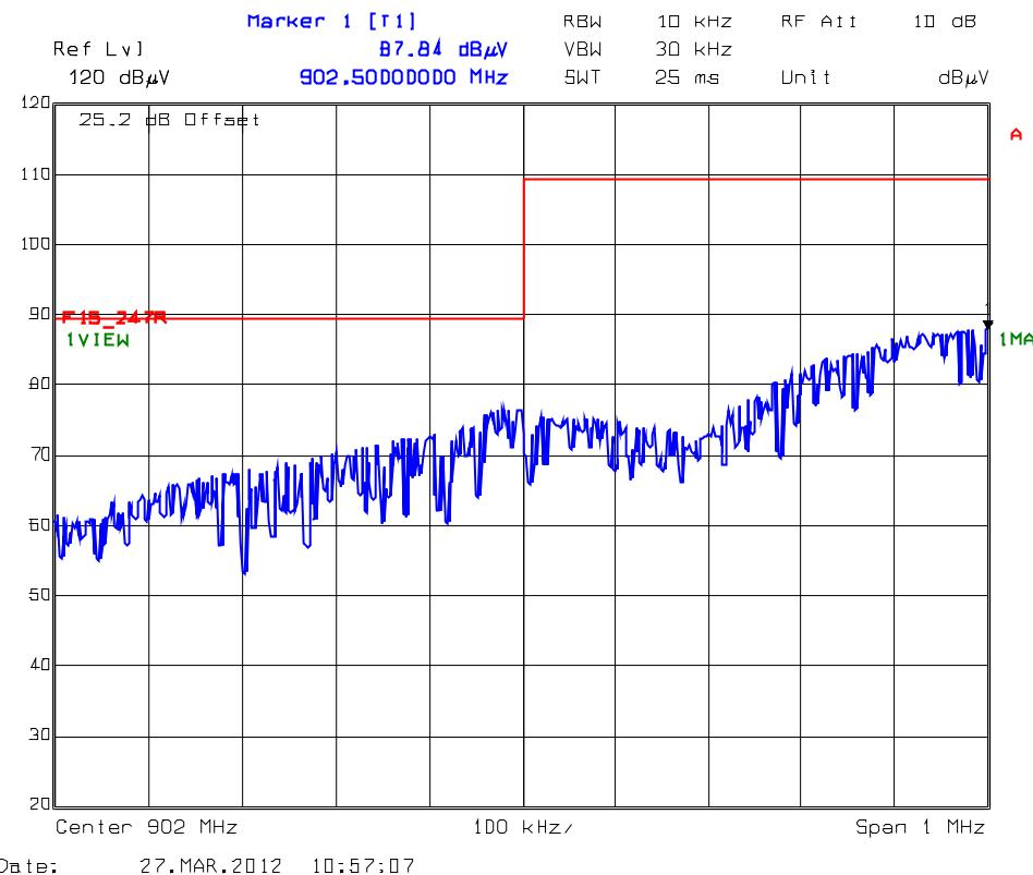
Lower Band Edge with Hopping Function ON
