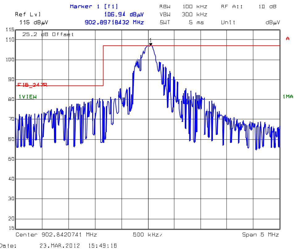
Lower Band Edge with Hopping Function ON
