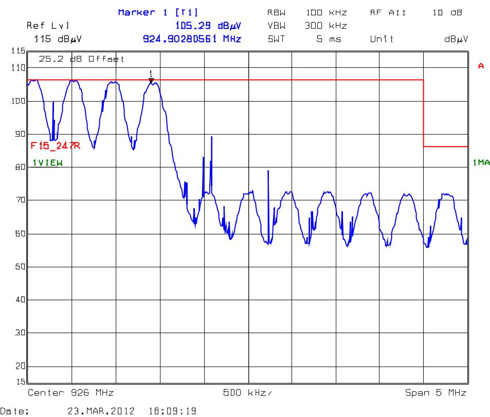
**Plot 5.10.4.1.4** Upper Band-Edge RF Radiated Emissions @ 3 meter
