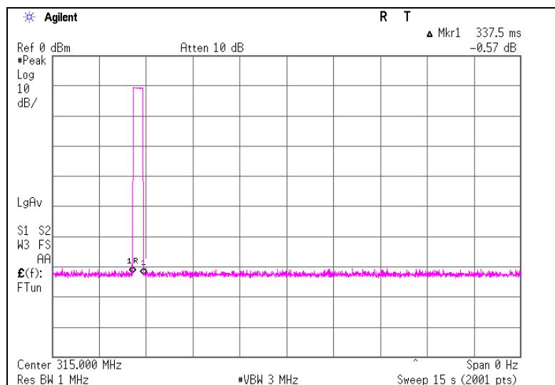
\* The EUT transmits UHF when LF signal is received from a car or a button on the EUT is pressed. In both cases, the UHF transmission is stopped within 5 seconds. So the test was performed by a button-pressed operation as the worst case. Please refer to the "Theory of Operation" for details.
