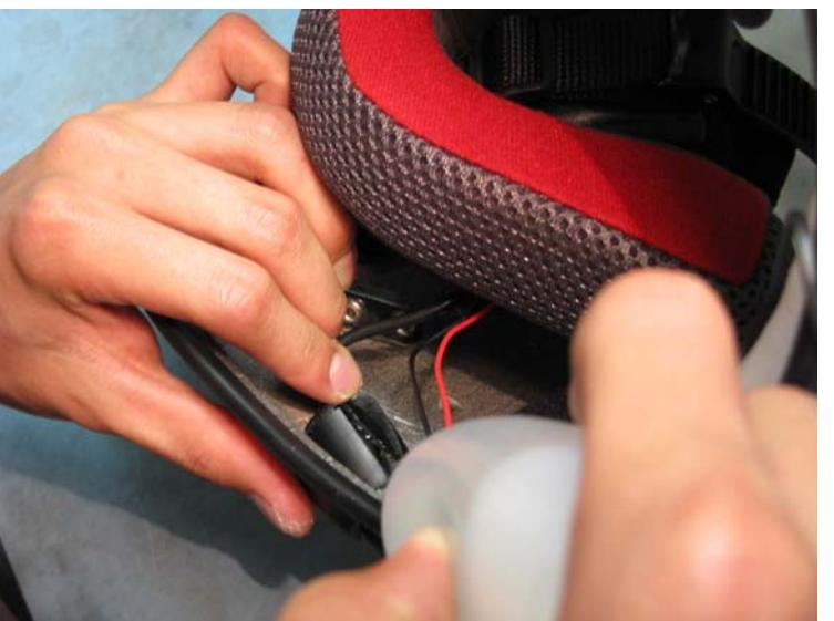
Glue the battery dc power wire in the rubber cap
