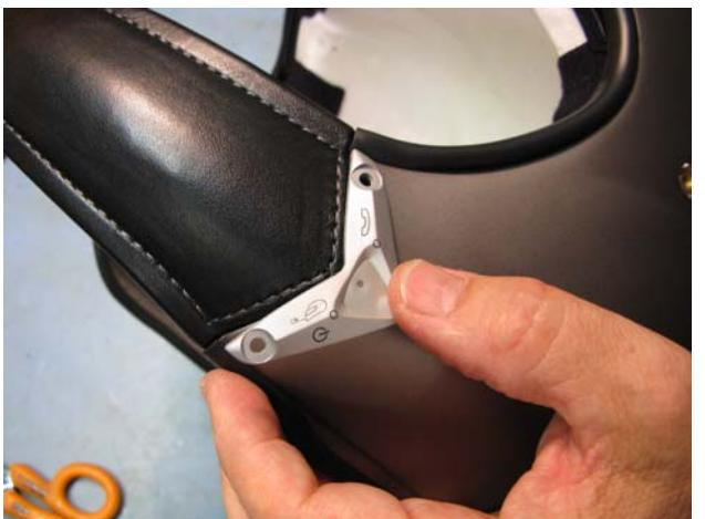
Place the key buttons, center it on the screw holes.
