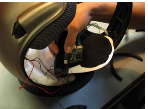
Place carefully the circuit in the correct place into the polystyrene part
