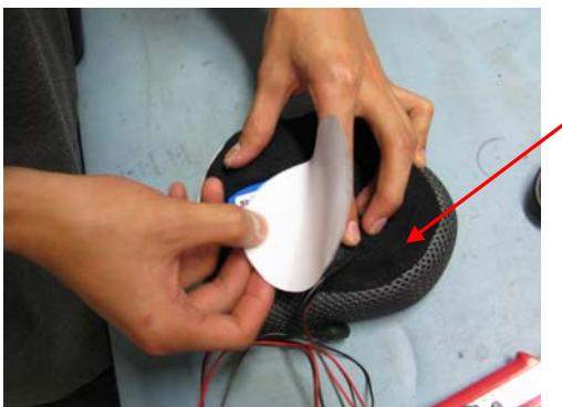
Cover the battery and wires with the sticky fabric
