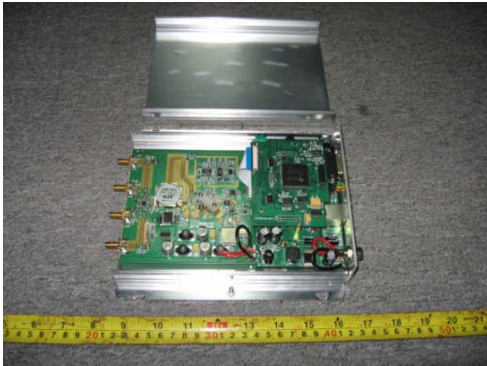
Photo 1- Uncovered view of EUT
