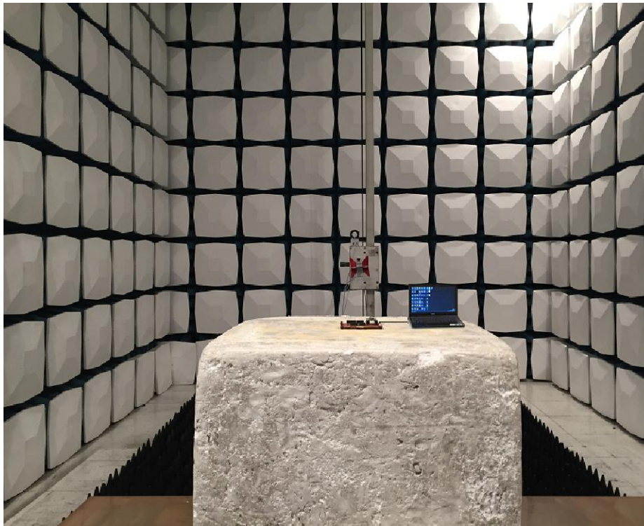
Description: Radiated Emission Test Setup for 1~18GHz
