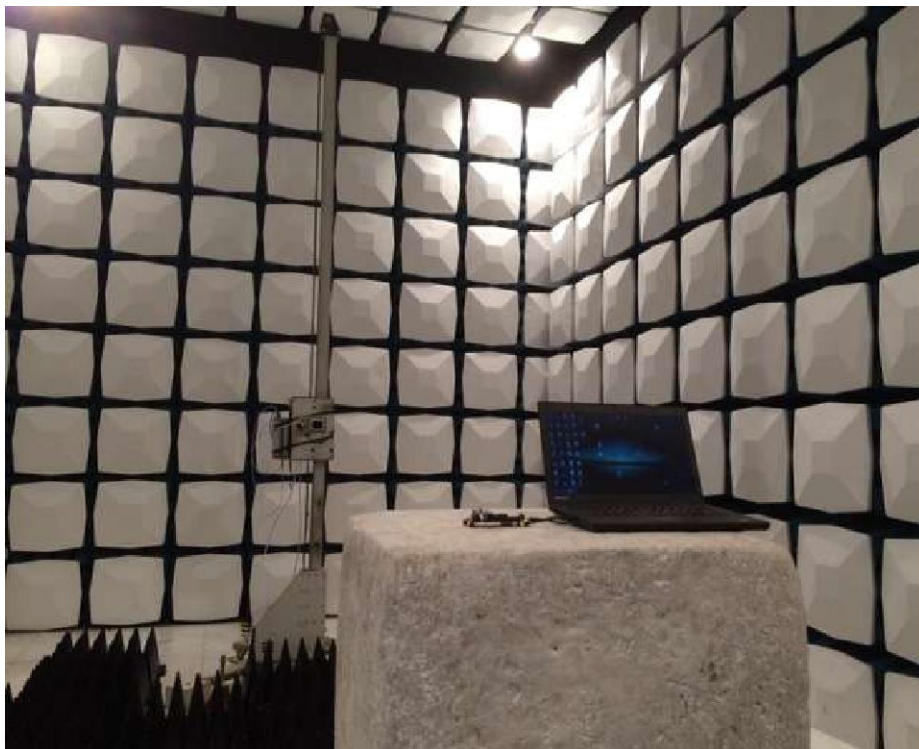
Description: Radiated Emission Test Setup for 18~40GHz
