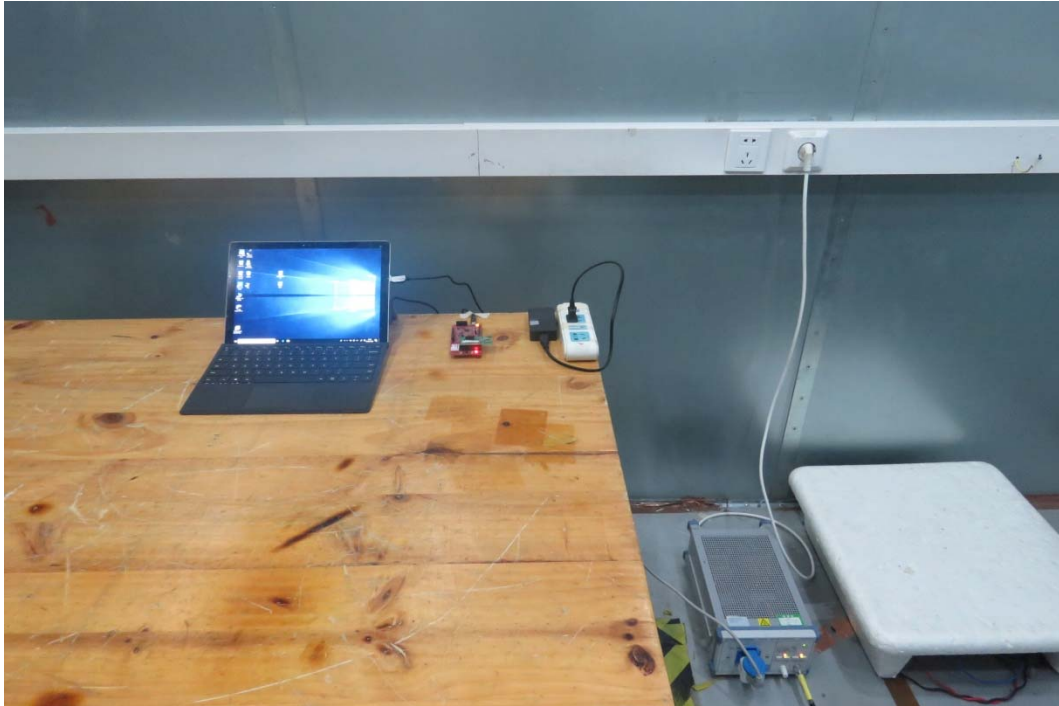
Picture 2 Conducted Emission Test Setup
