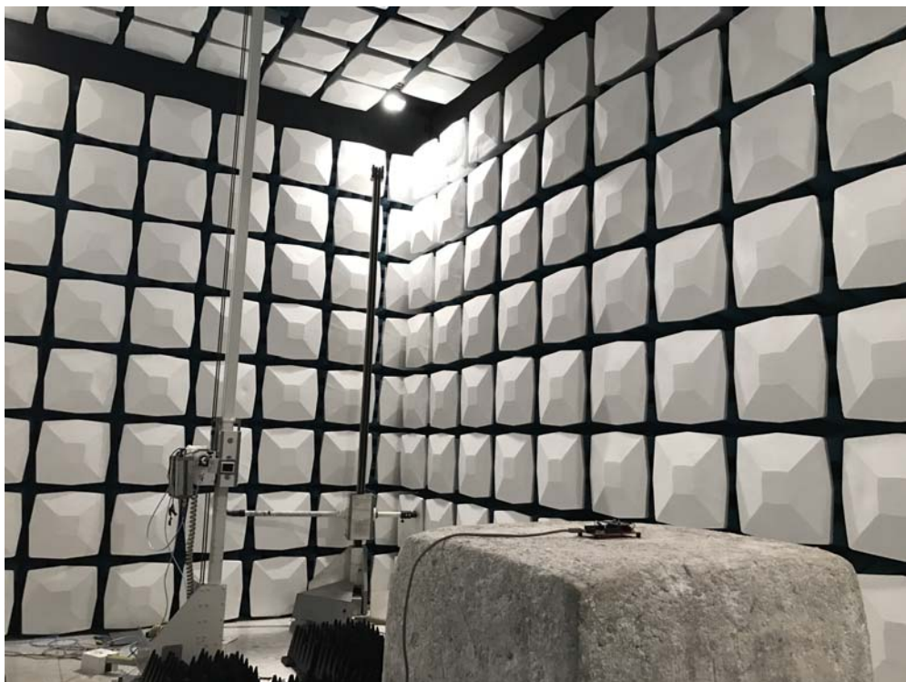
Description: Radiated Emission Test Setup for 18~40GHz
