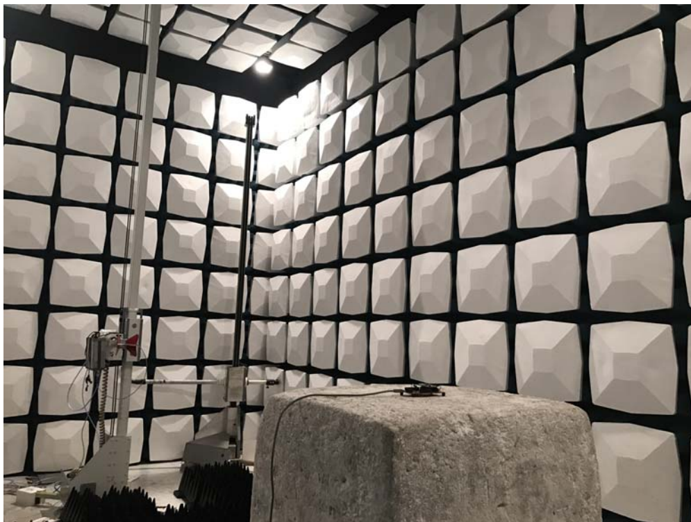
Description: Radiated Emission Test Setup for 1~18GHz
