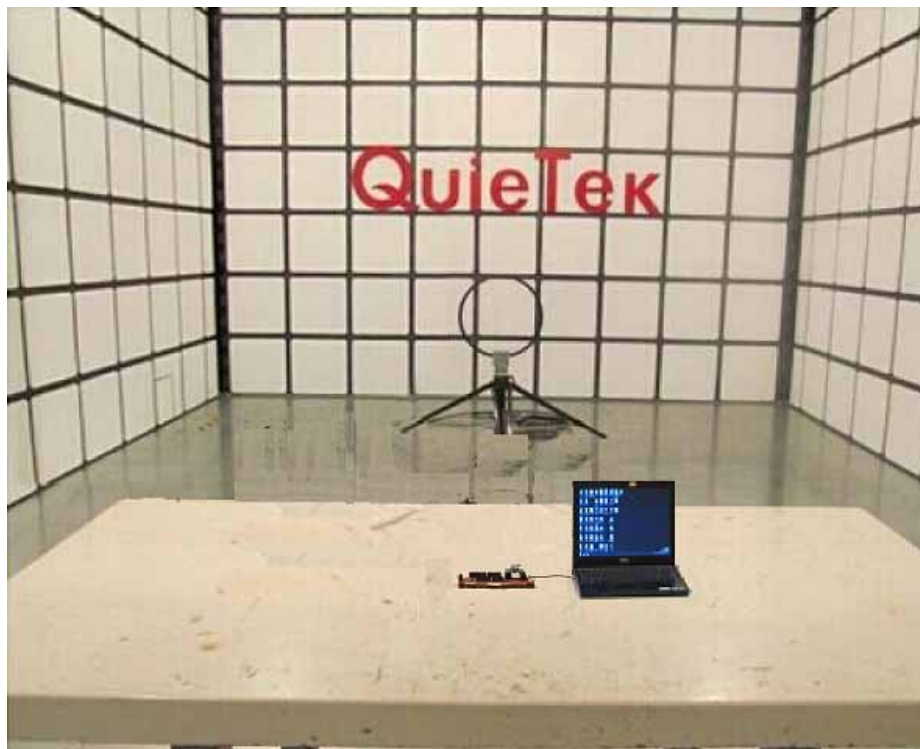
Description: Radiated Emission Test Setup for Below 30MHz
