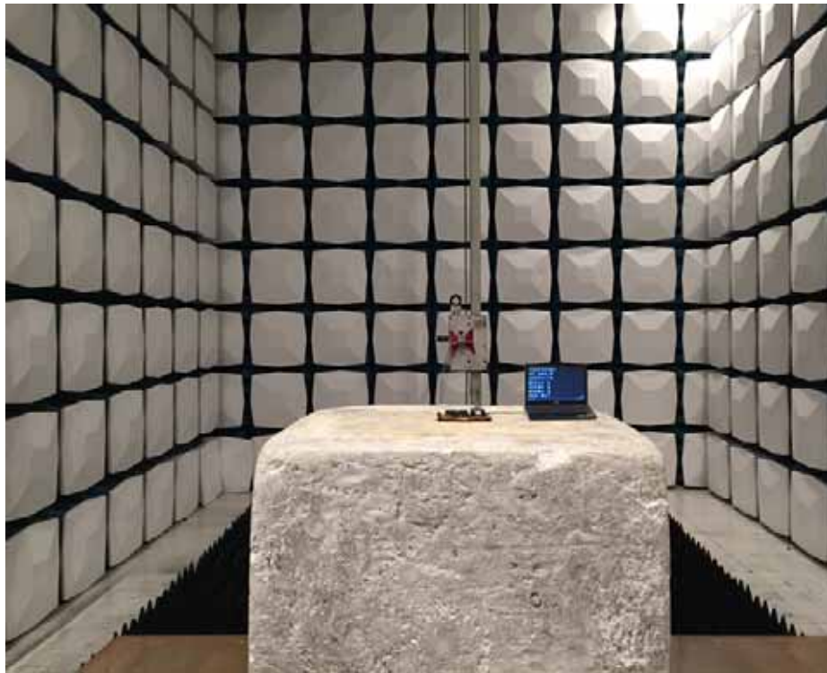
Description: Radiated Emission Test Setup for 1~18GHz
