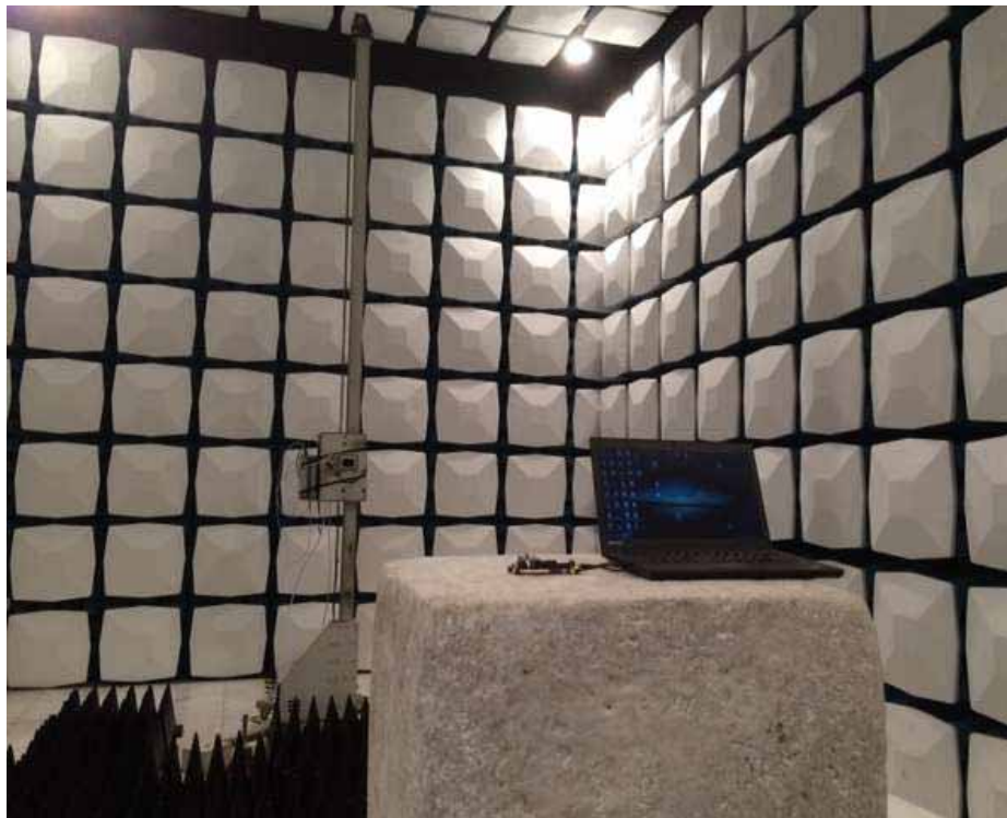
Description: Radiated Emission Test Setup for 18~40GHz
