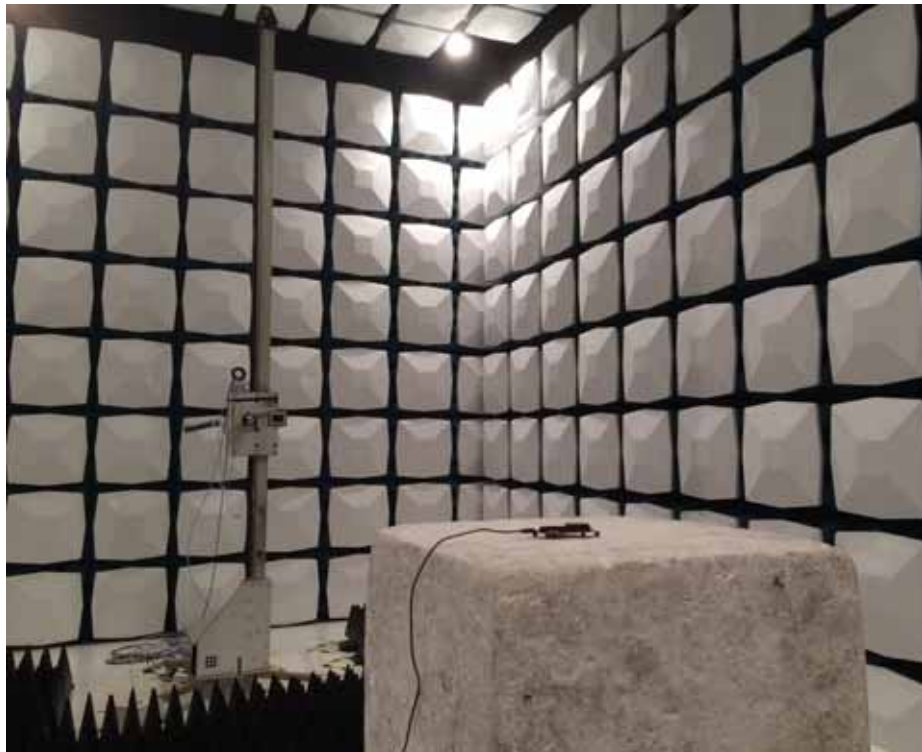
Description: Radiated Emission Test Setup for 18~40GHz
