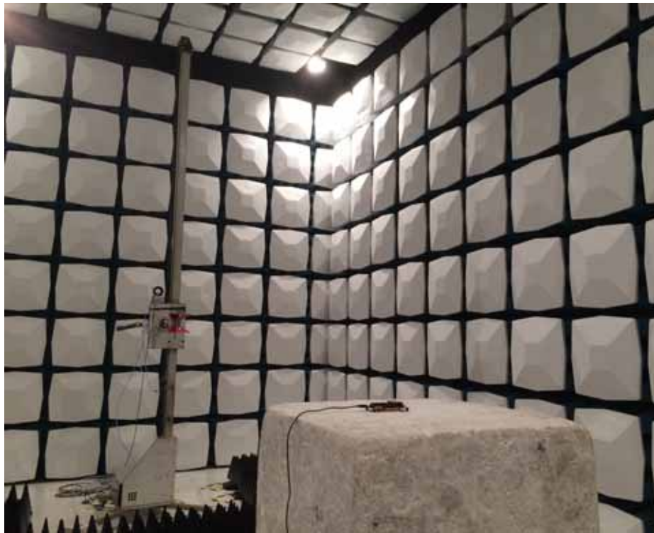
Description: Radiated Emission Test Setup for 1~18GHz
