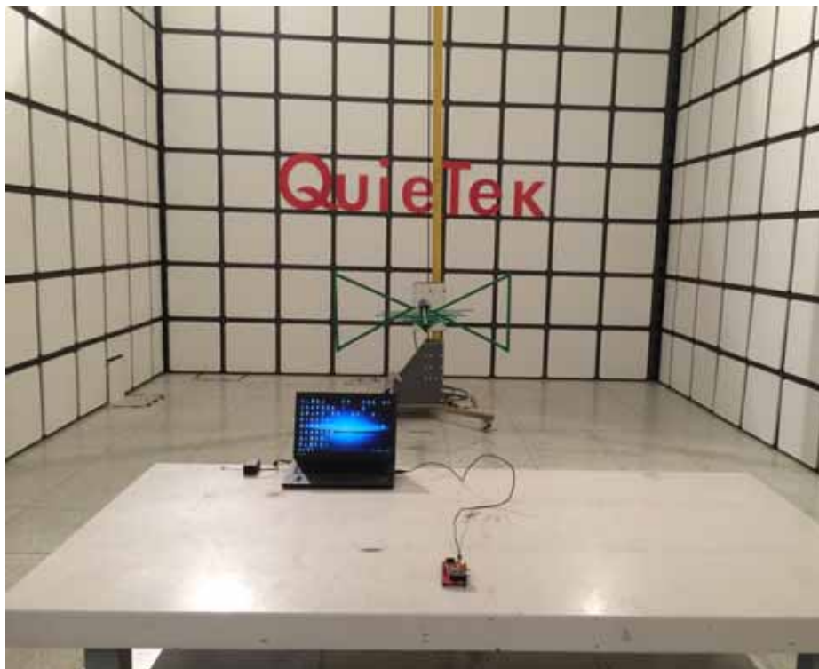
Description: Radiated Emission Test Setup for Below 1GHz
