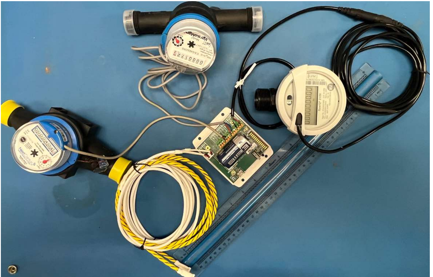
Uncovered AquaLink connected to 2 pulse meters, 1 encoded meter and 2 rope sensors
