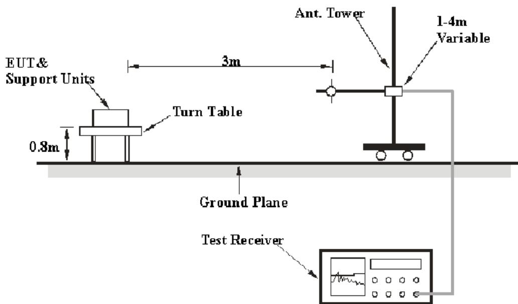
The radiated emission tests were performed in the 3-meter chamber a test site, using the setup accordance with the ANSI C63.4-2009. The specification used was the FCC Part Subpart C limits.
