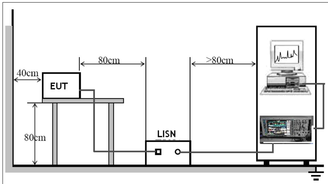
The EUT was placed on the test table in shielding room
