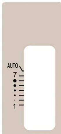
1. When the lever is in AUTO position, the printer will measure the paper thickness before printing and then automatically adjust the gap between the print head and the paper.
