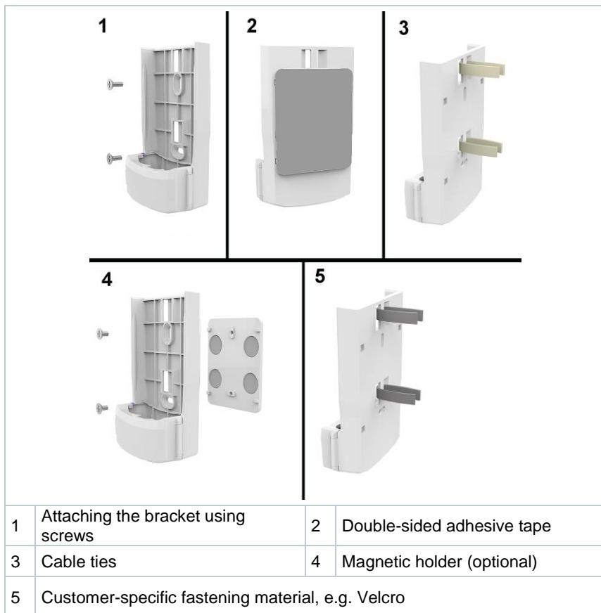
1 | Mount the wall bracket at the designated location using suitable mounting materials.
