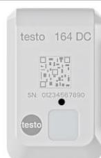
The testo 164 DC is an easy-to-use online data logger for monitoring doors (opening & closing).
