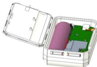
4 Remove the circuit board and battery (red arrow) and dispose of them separately in accordance with local regulations.
