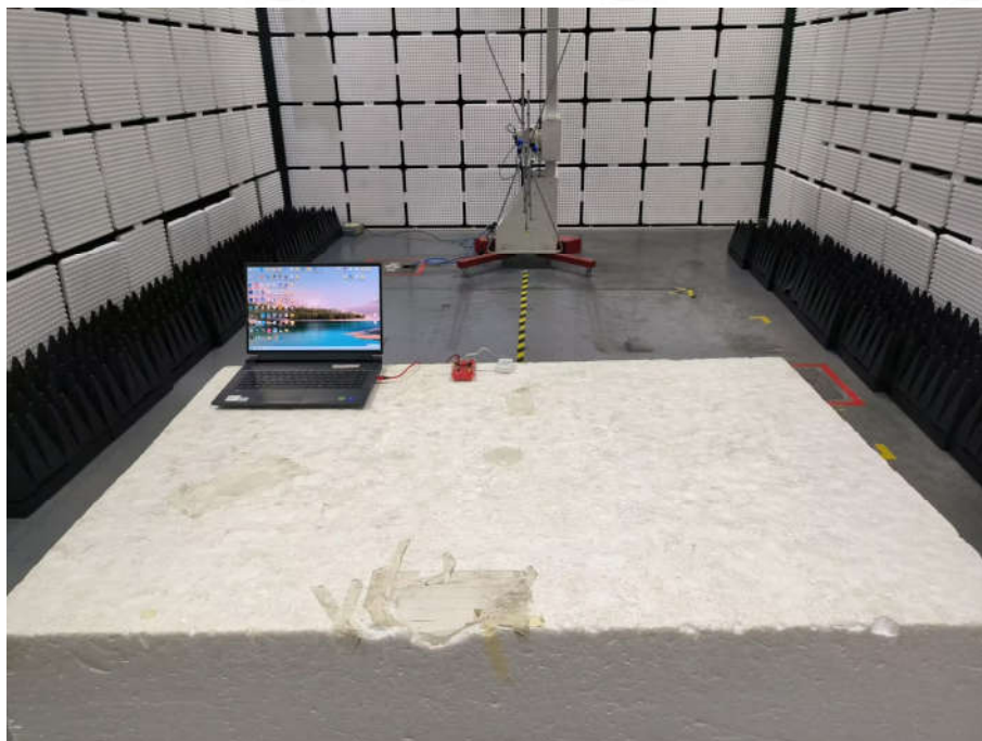
Radiated spurious emission Test Setup-1(Below 1GHz)
