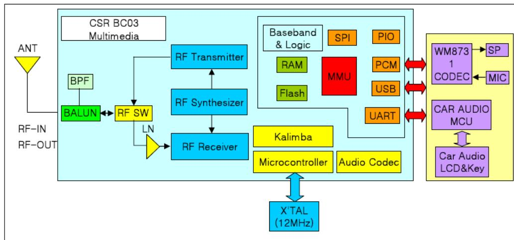
The RF transceiver/reciever circuit is composed of NBM2XA -XX and its accessory components.
