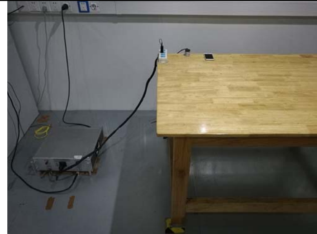
Conducted Emissions Test Setup Front View
