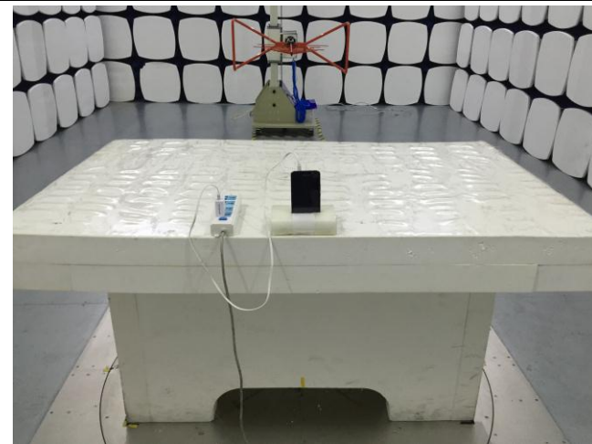
Conducted Emissions Test Setup Front View
