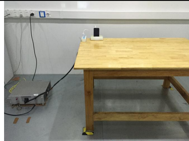
Conducted Emissions Test Setup Front View
