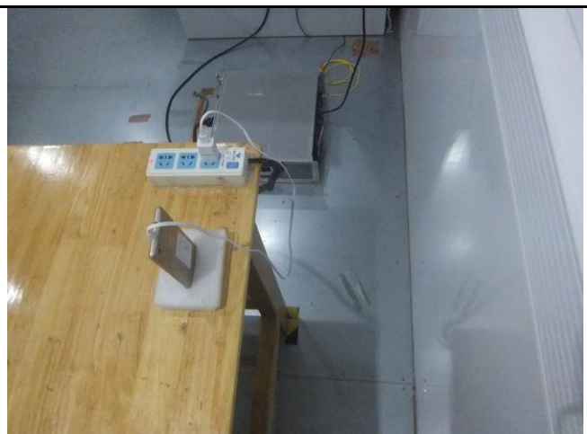
Conducted Emissions Test Setup Side View
