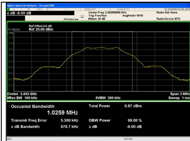
6dB Bandwidth - Low CH 2402
