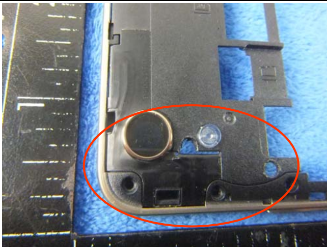
LTE - Antenna View
