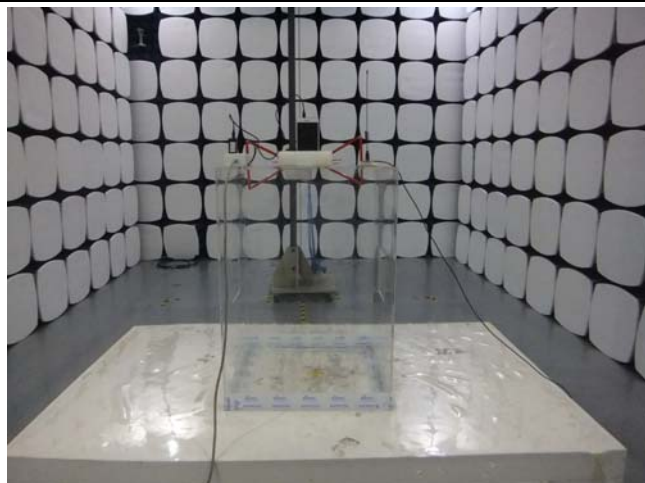
Radiated Spurious Emissions Test Setup Below 1GHz
