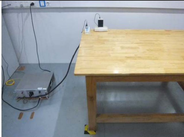
Conducted Emissions Test Setup Front View
