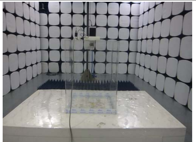
Radiated Spurious Emissions Test Setup Above 1GHz
