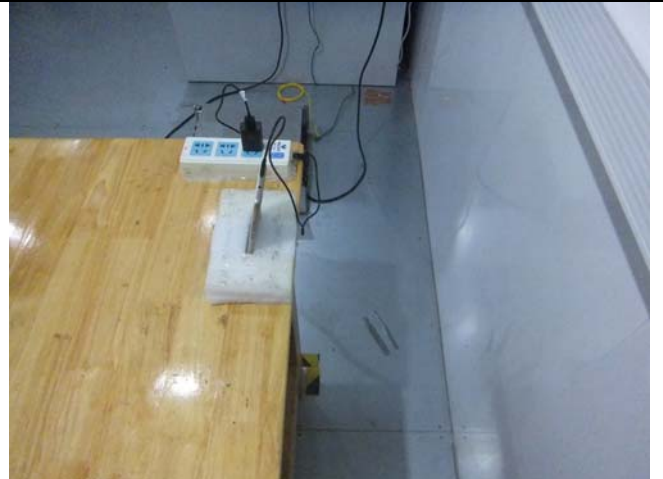
Conducted Emissions Test Setup Side View
