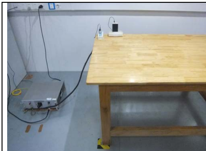
Conducted Emissions Test Setup Front View
