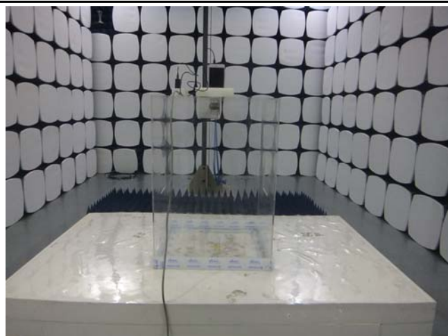
Radiated Spurious Emissions Test Setup Above 1GHz
