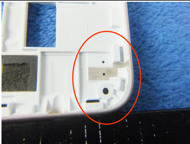
LTE - Antenna View
