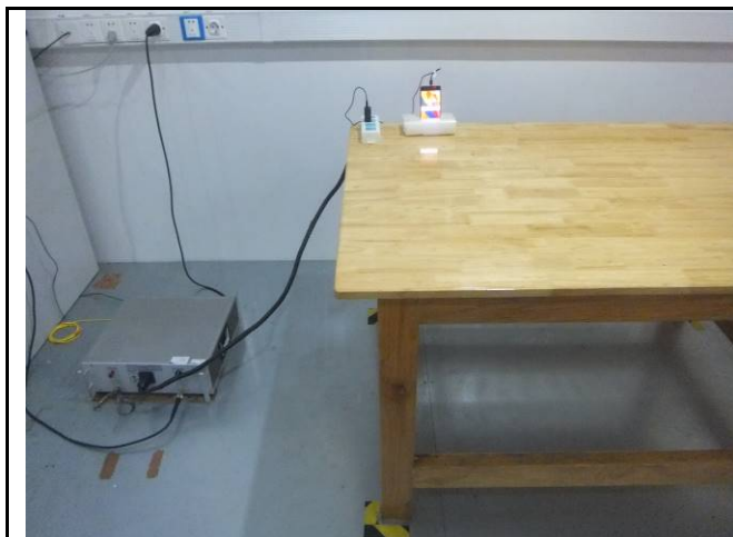
Conducted Emissions Test Setup Front View
