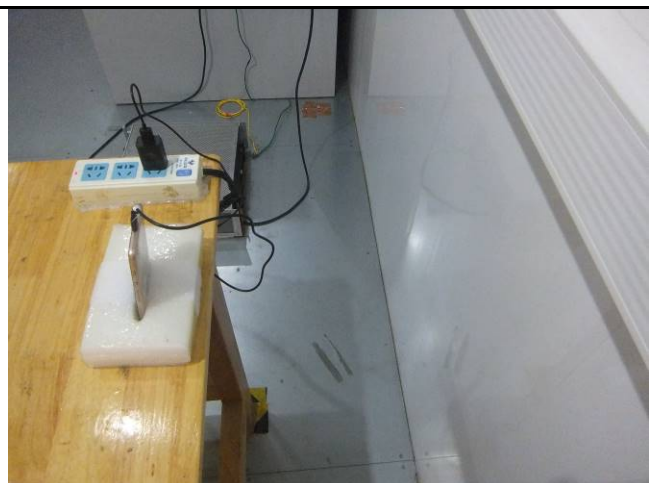
Conducted Emissions Test Setup Side View
