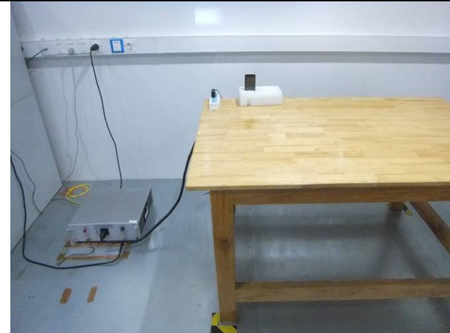
Conducted Emissions Test Setup Front View
