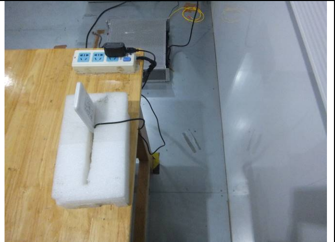
Conducted Emissions Test Setup Side View
