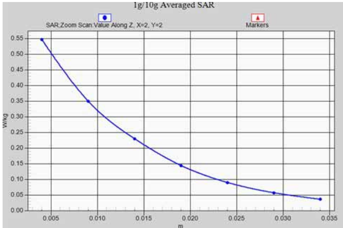
GPRS 1900/Back side-Mid _ z-axis scan
