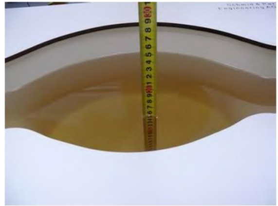
Liquid depth in the body phantom (835MHz)
