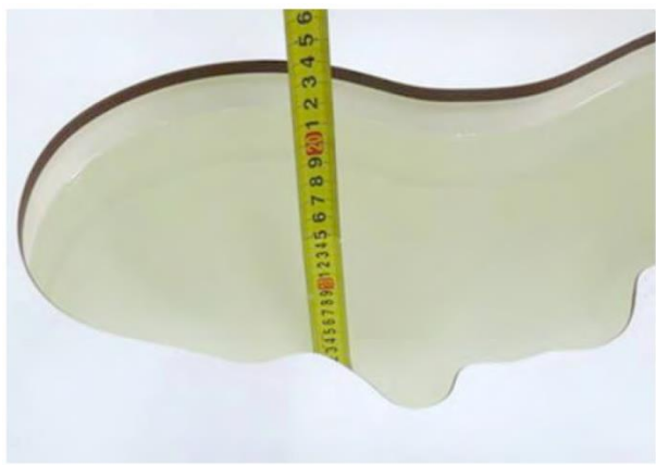
Liquid depth in the head phantom (1900MHz)
