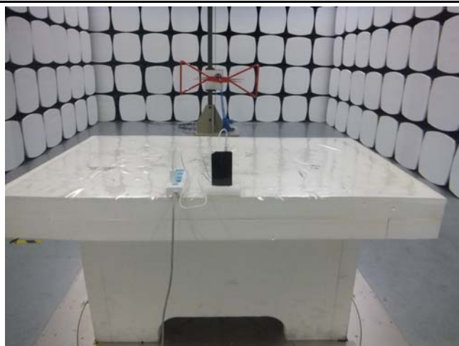
Conducted Emissions Test Setup Front View
