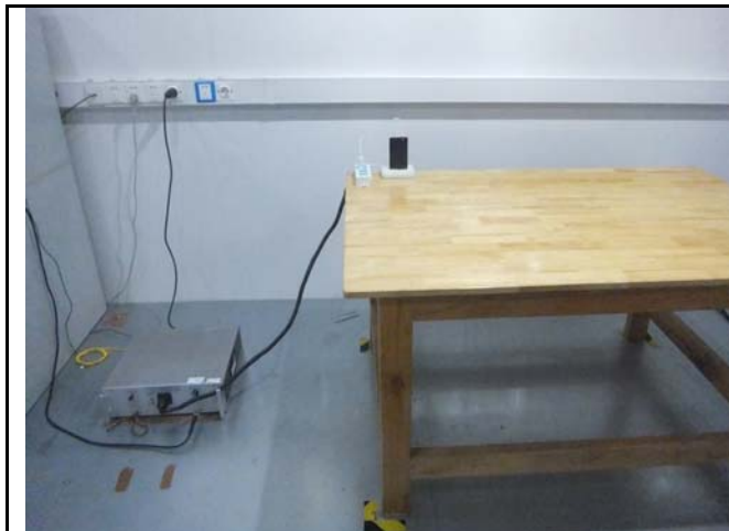
Conducted Emissions Test Setup Front View
