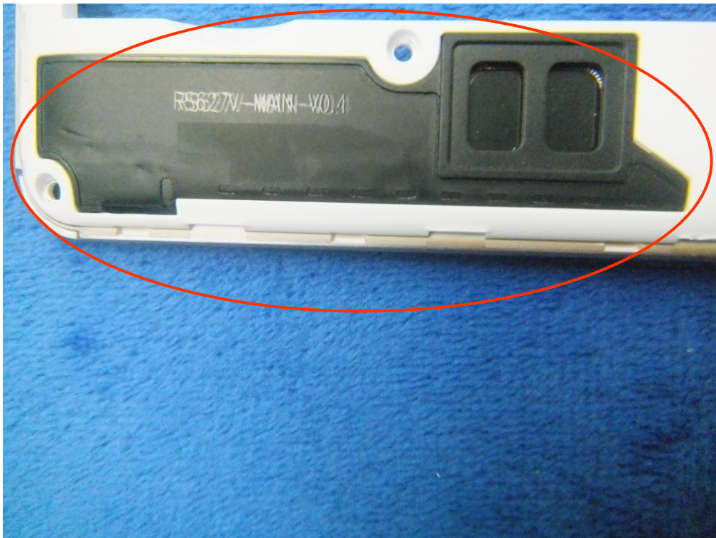
GSM/PCS/UMTS - Antenna View
