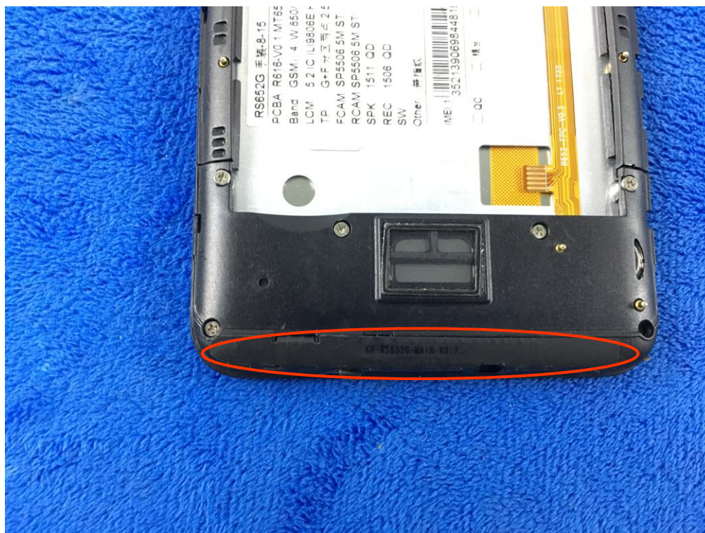
GSM/PCS/UMTS-FDD Antenna View
