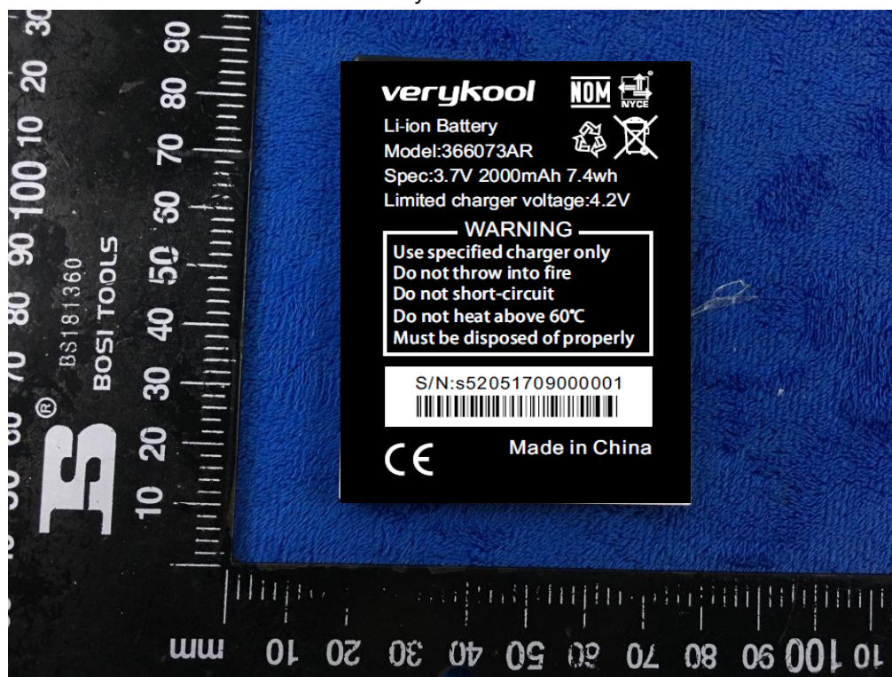
Battery - Front View
