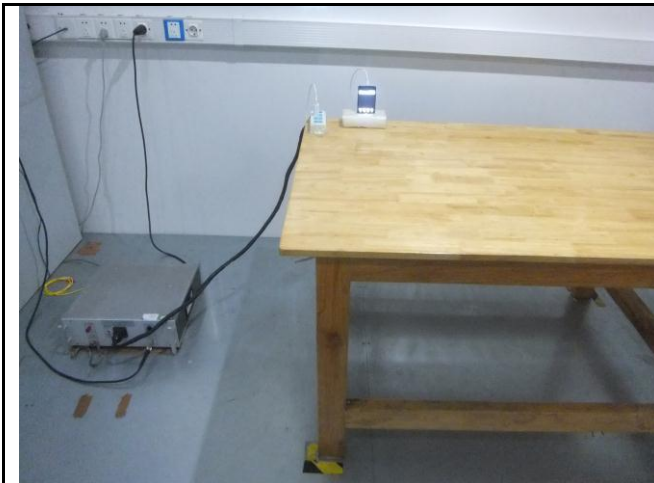
Conducted Emissions Test Setup Front View
