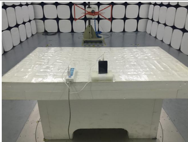
Conducted Emissions Test Setup Front View
