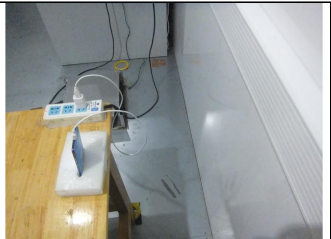
Conducted Emissions Test Setup Side View
