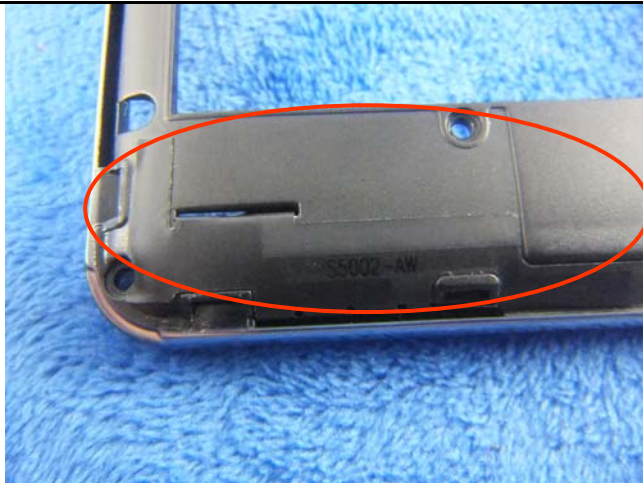
GSM/PCS/UMTS-FDD Antenna View
