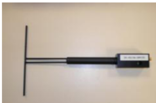
Figure 1 – Satimo COMOSAR Validation Dipole
