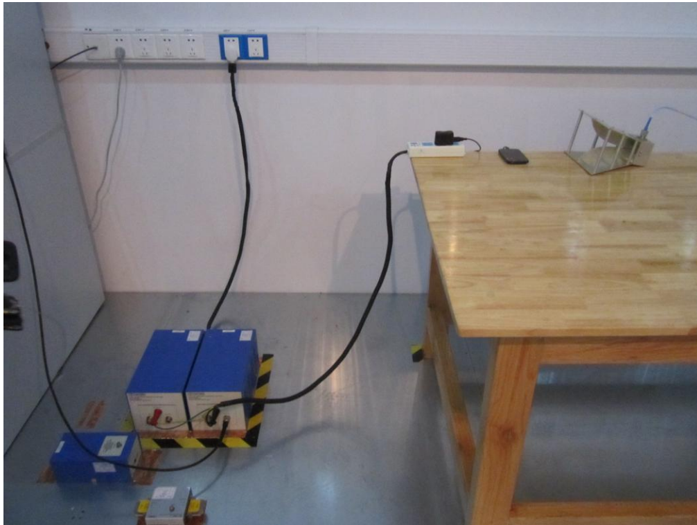
Conducted Emissions Test Setup Front View
