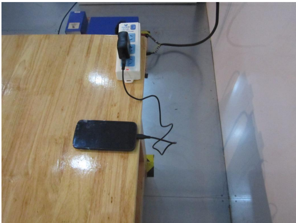
Conducted Emissions Test Setup Side View
