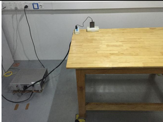
Conducted Emissions Test Setup Front View
