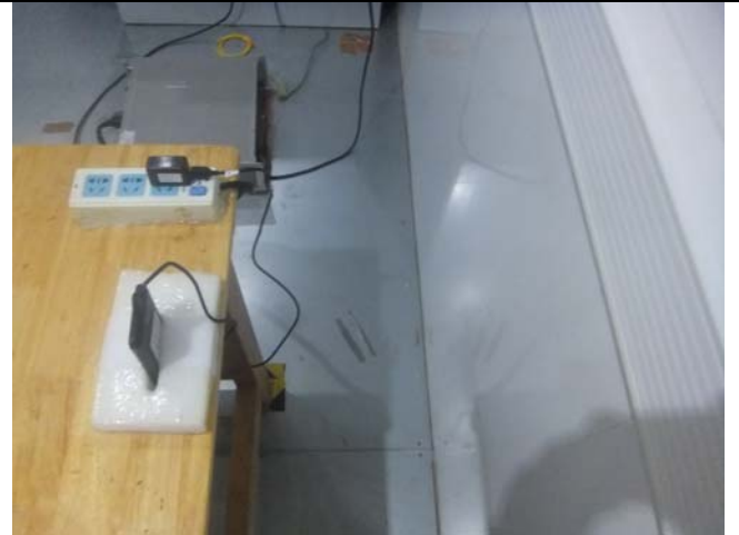
Conducted Emissions Test Setup Side View
