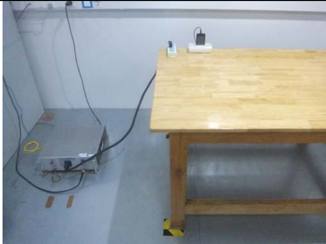
Conducted Emissions Test Setup Front View
