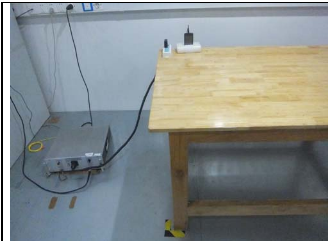
Conducted Emissions Test Setup Front View
