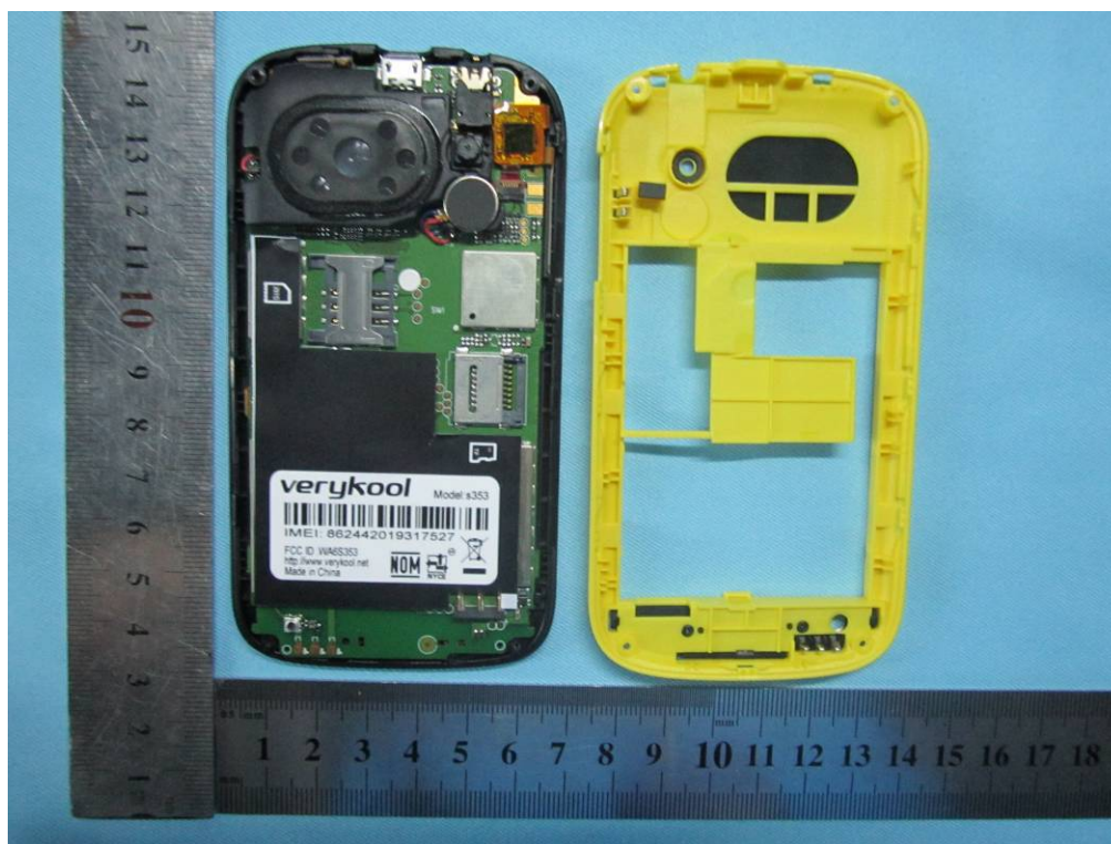
Cover Off - Rear Housing View type B (one SIM card)
