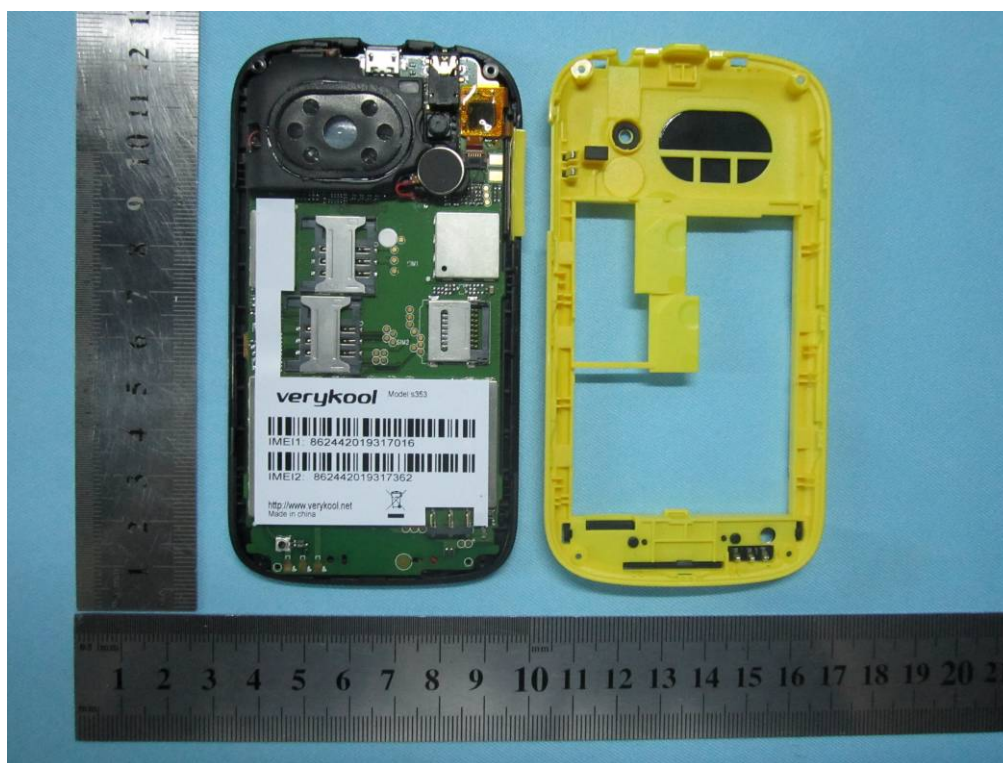
Cover Off - Rear Housing View type A (two SIM card)
