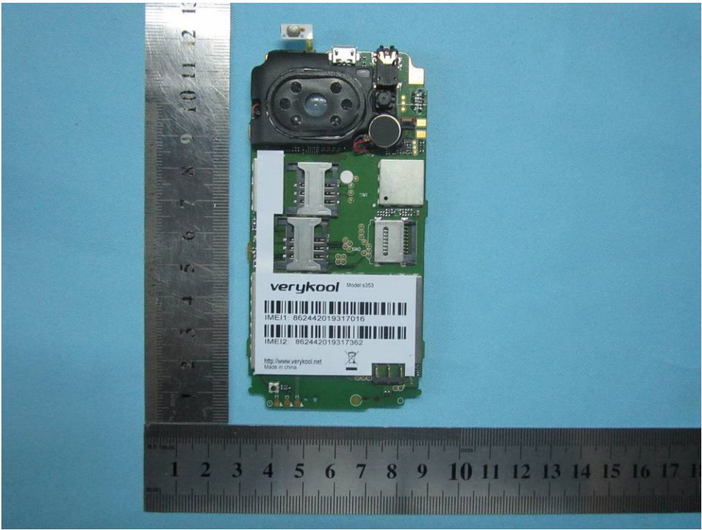
Mainboard With Shielding - Front View
