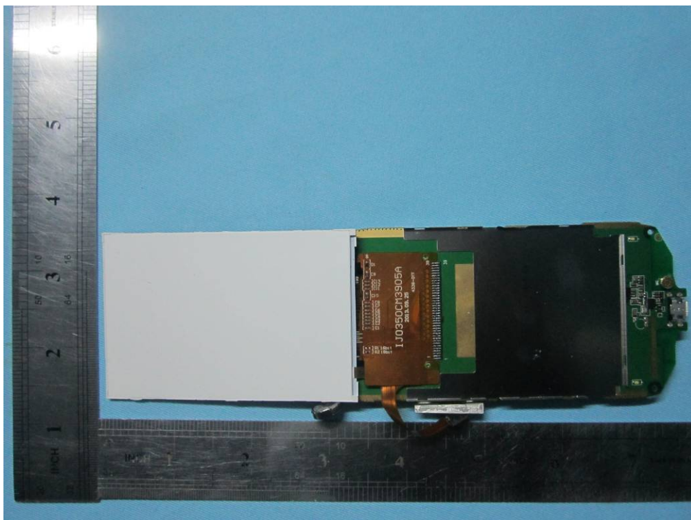
Mainboard Without Shielding – Rear View
