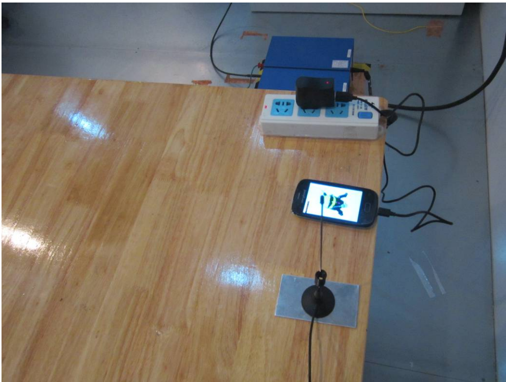
Conducted Emissions Test Setup Side View
