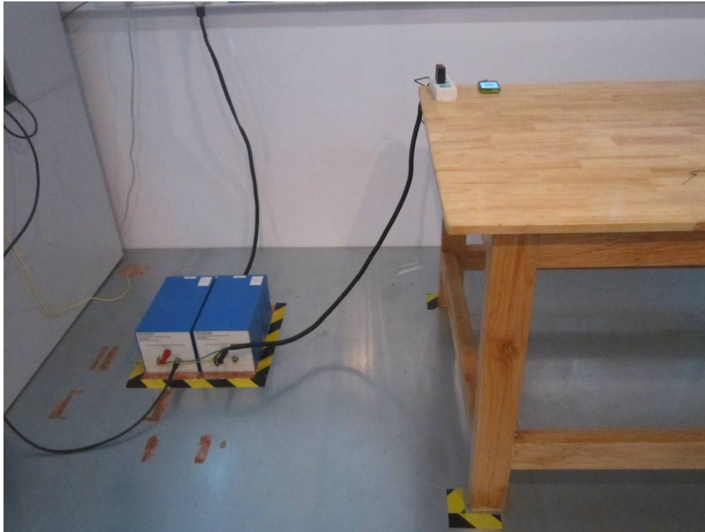
Conducted Emissions Test Setup Front View
