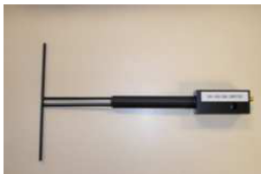
Figure 1 – Satimo COMOSAR Validation Dipole
