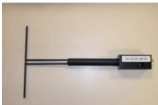
Figure 1 – Satimo COMOSAR Validation Dipole
