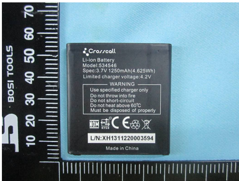
Battery - Top View
