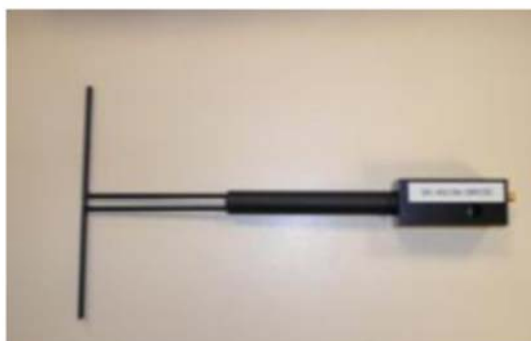
Figure 1 – Satimo COMOSAR Validation Dipole
